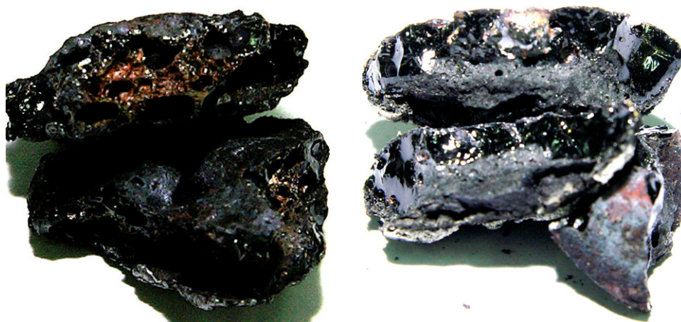
Fig. 2. The sections of the sinters made from synthetic sludge with iron powder by microwave sintering (left) and by improved microwave sintering (right) at 800 W for 30 min.
